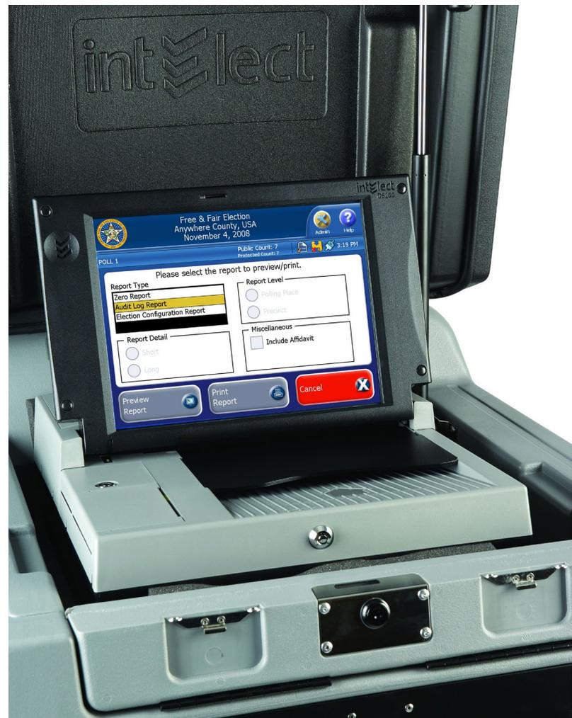
a connection that it did not initiate. Results are sent over a secure and hardened network. Static Internet Protocol (IP) addresses are assigned to the modem inside each DS200. These IPs are added to the server's "white list" while all other incoming IP addresses are blocked for a secure transfer.
